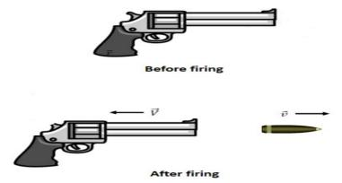
Based on this principle, we are able to explain the recoiling of a gun when a bullet is fired, flights of jet planes and rocket, Explosion on bomb etc. in all these cases if one part of system is moving in one direction then the other part move in such a direction that total linear momentum may remain constant.
